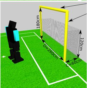
Yellow goalposts and crossbar made from cylinders with a diameter of 10cm (approx. 4 inches). The crossbar is in 180cm height.
