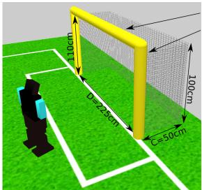
Goalposts and crossbar made from 3 yellow cylinders with a diameter of 10cm (approx. 4 inches). The crossbar is in 110cm height.
